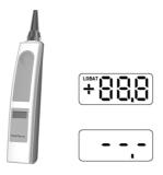
Press the start button again to start the measuring process. The measuring cycle consists of 16 impulses of the pressure sensitive tapping head against the measuring object (tooth, implant). For each valid impulse a low tone is emitted. Invalid impulses, for example due to a too high deviation from the correct posture of the Periotest M, are followed by a high tone. You can correct the posture of the Periotest M during the measuring process.
